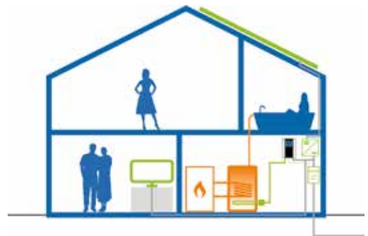
Photovoltaic water heating up to 9 kW
